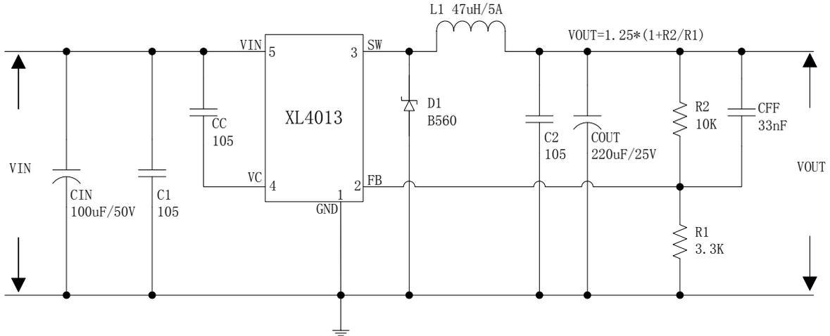
Figure5. XL4013 System Parameters Test Circuit (VIN=8V~36V, VOUT=5V/4A)
