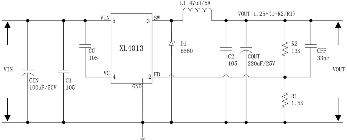
Figure7. XL4013 System Parameters Test Circuit (VIN=15V~36V, VOUT=12V/3A)
