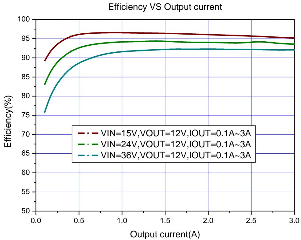
Figure8. XL4013 System Efficiency Curve
